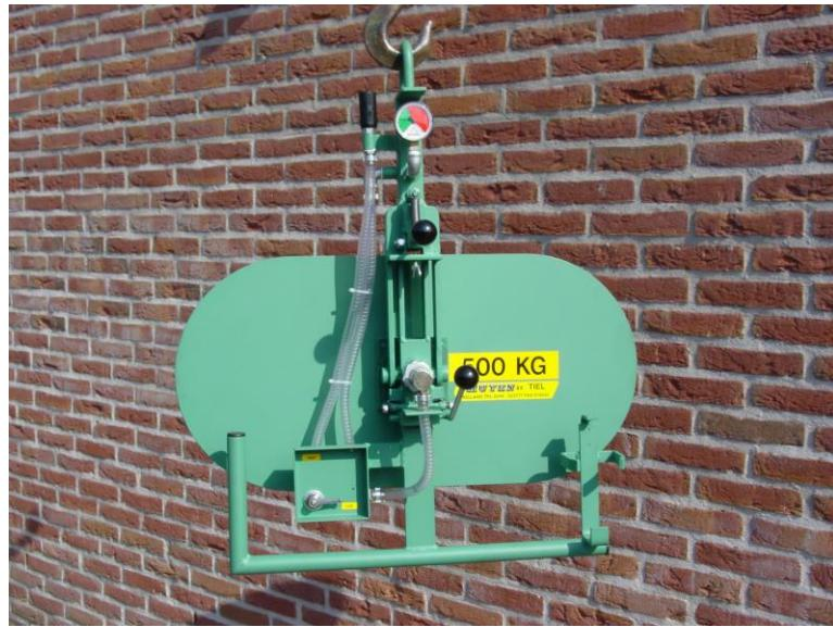
**This vacuummachine works with a vacuum pump that has a built in crane or swivel arm that is suitable for internal transport of glass and other sheet material with a flat surface and dense structure.**
